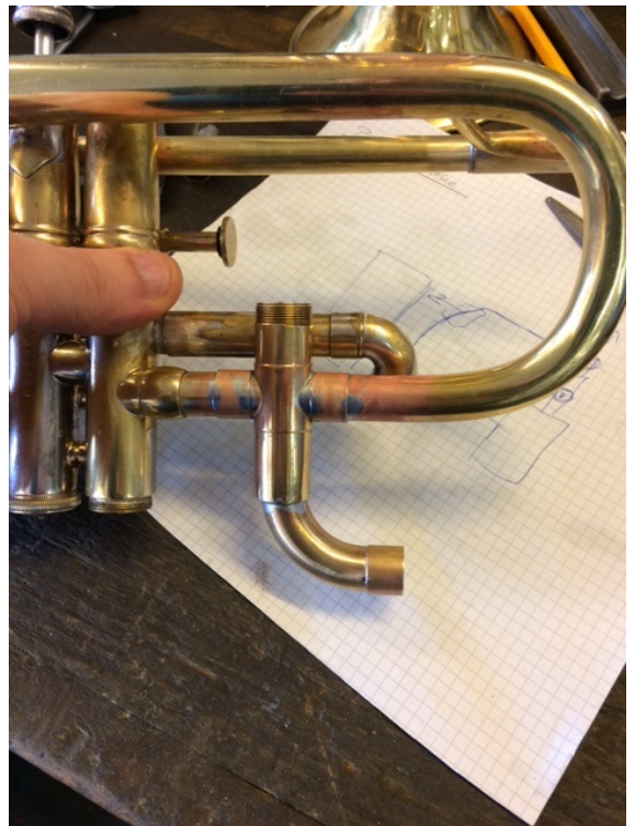
Preparing to install the switch valve
