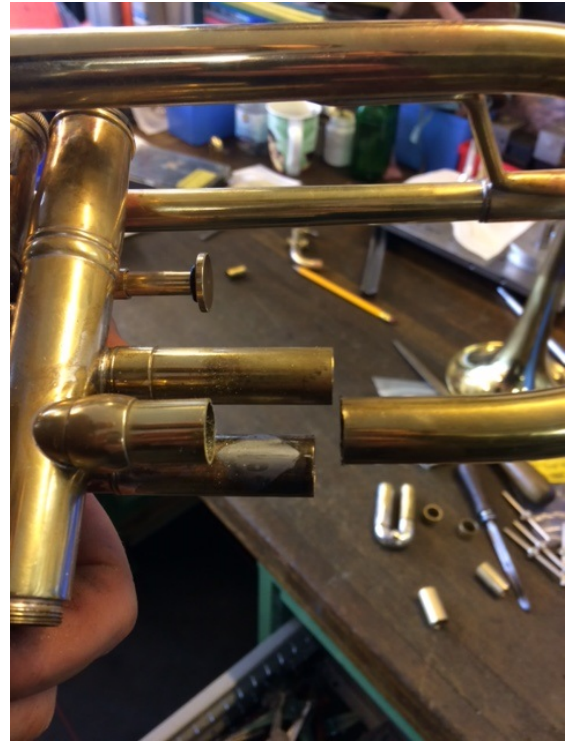
Preparing to install the switch valve
